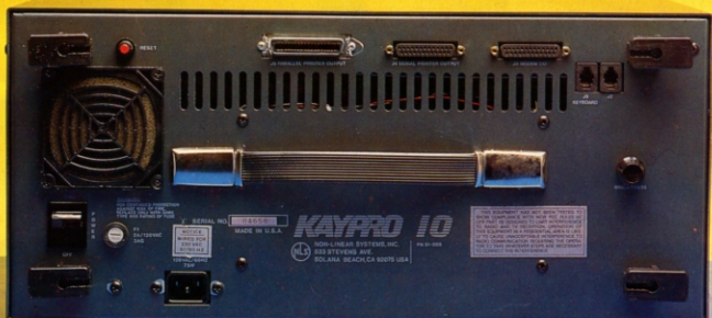
The top of the system packed for portability — around the handle are clustered ports, a vent and superfluous feet. Below, the stylish Kaypro 10 dashboard.
